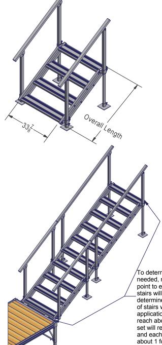
To determine length of stairs needed, measure from start point to end point of where stairs will be needed, then determine what combination of stairs will best suit your application. A 4 step set will reach about 4 feet, a 6 step set will reach about 6 feet, and each splice kit adds about 1 foot of length.
