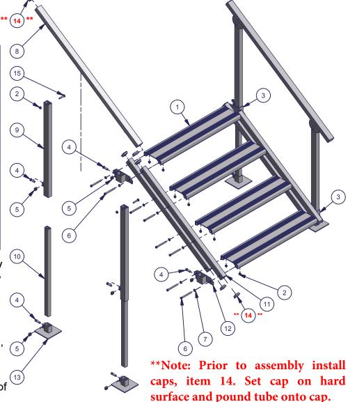
step drilled tubes. Set cap on hard surface and pound tube onto cap.
