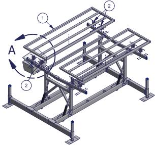
Step 2. Slide the Bunk Brackets onto the Lift Rack Beam. Fasten to the Float Plane Platforms with one 3/8" x 3-1/4 Hex Bolt and 3/8" Flanged Hex Nut at each connection point.
