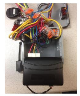
Carefully move the black remote box to an easy to work with position and separate the cover from the black box by gently removing top from bottom.
