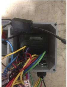
Once the cover is off the box, carefully move the wires out of the way to reveal the antenna and black remote box.
