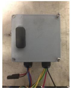
Remove the four screws from the control box cover.
