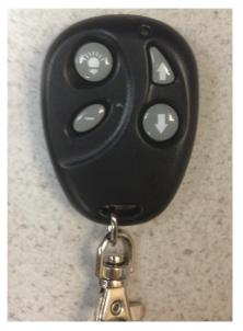
Upper right button is the "UP" button. Upper left button is for the canopy light. Bottom right button is the "DOWN" button.
