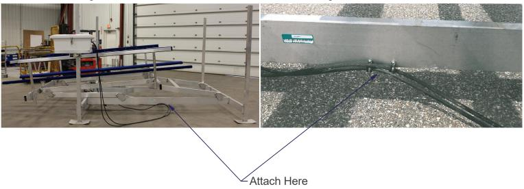
Do not attach hoses to lift between lift sides or to H-Frame. When lift rises they will get pulled off. Attach to lift sides only.
