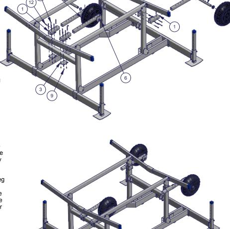
Step 4. When rear leg pockets are in desired location, slide the rear wheel legs into the leg pockets with the wheel facing out for greater stability. Secure the wheels at desired height by inserting a J-pin through the adjustment holes in the leg pocket and wheel leg. Make sure all wheels are in desired location and all hardware is tightened.
